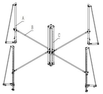
A. Triangle Out Rigger B. Rail C. Centre piece
